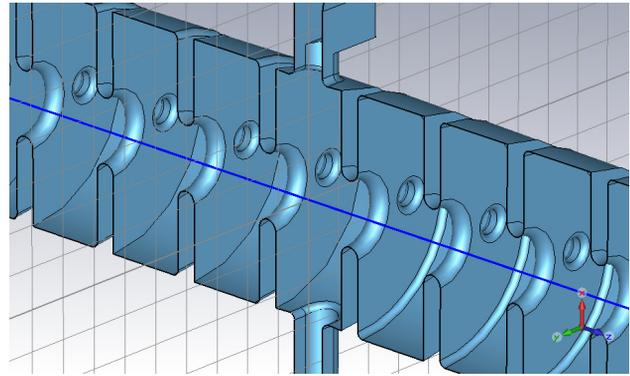
Figure 6: Cut-plane view of the cell-shapes and coupler design.
