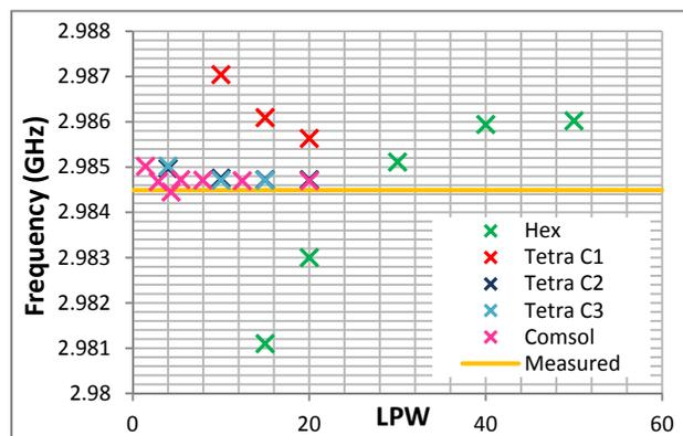
Figure 4: Frequency comparison between hexahedral and tetrahedral meshes, at different orders of curvature.
