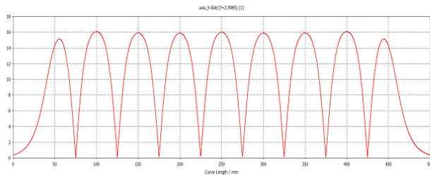
Figure 5: Simulated field flatness of the magnetic field in the final 9-cell cavity.
