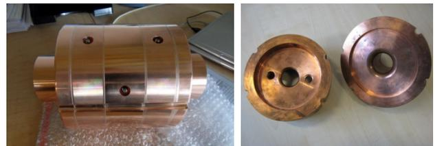
Figure 2: Prototype 3-cell cavity and sections.
