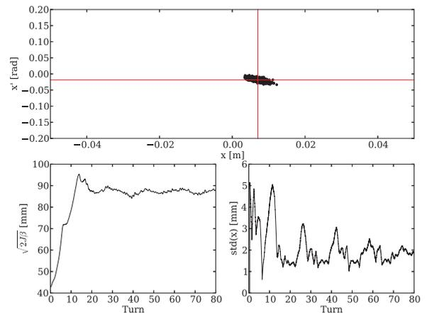
Figure 3: Initial transverse phase space evolution for the simulation in figure 2 (b). The red cross-hair represents the mean. The bottom left panel shows the mean betatron amplitude of the bunch. The bottom right panel shows the standard deviation of the horizontal coordinate.
