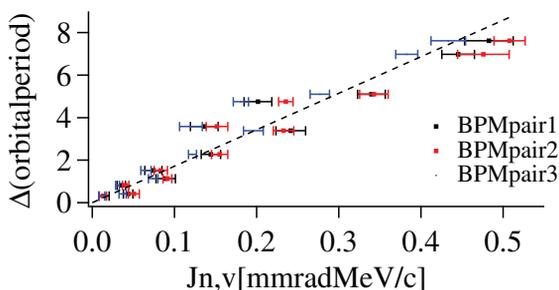
Figure 5: Change in orbital period vs. vertical transverse action. Dashed line is from theory.
