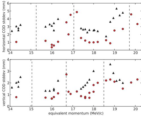
Figure 1: COD before (black triangles) and after (red circles) correction in the horizontal (top panel) and vertical (bottom panel) planes over the momentum range. The vertical dashed lines indicate the approximate location of integer tunes.
