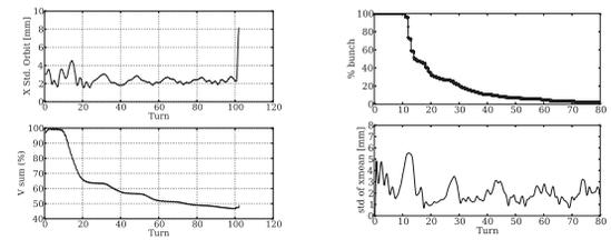
Figure 2: (a) shows the standard deviation of the horizontal BPM measurement and the charge reduction for an experiment in EMMA. (b) shows the same parameters for a bunch simulated in pyZgoubi with a magnetic model and bunch distribution approximately the same as the experiment. The beam is placed in a synchrotron bucket with 0.5 MV/turn acceleration.
