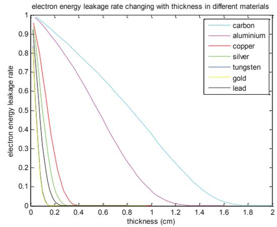
Figure 5: electron energy leakage rate changing with thickness in different materials.
