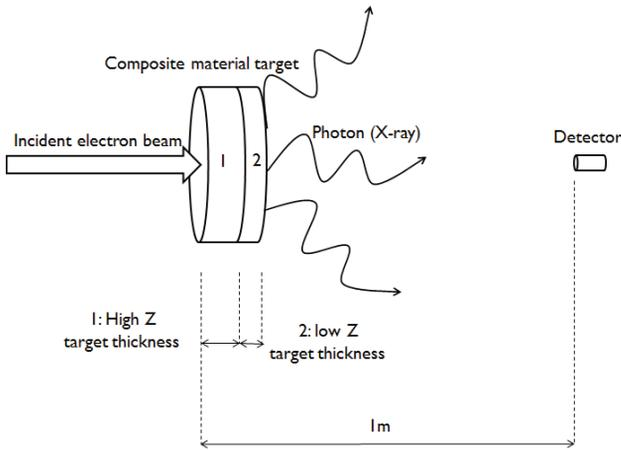
Figure 3: Composite material target model.
