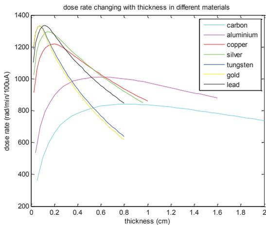
Figure 4: dose rate changing with thickness in different materials.
