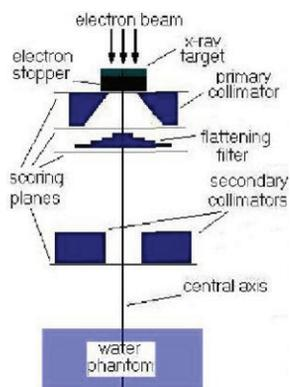
Figure 1: Schematic representation of the simulated Clinac 2300EX treatment head [2].
