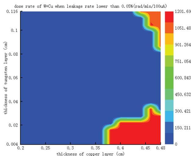
Figure 7: dose rate of W+Cu composite material target when electron energy leakage rate is lower than 0.05%.
