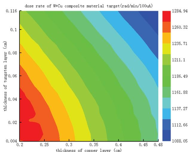
Figure 6: dose rate of W+Cu composite material target.
