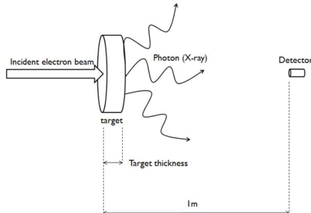
Figure 2: Single material target model.
