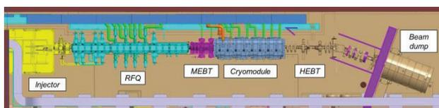
Figure 1: General layout of the LIPAc accelerator.
