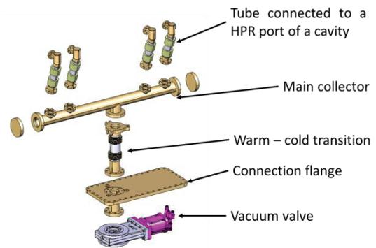
Figure 6: The vacuum manifold.
