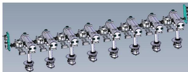
Figure 2: The cavity string of the cryomodule.
