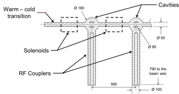
Figure 3: section view of the first elements of the cavity string.
