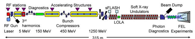
Figure 1: Schematic layout of the FLASH facility [2].
