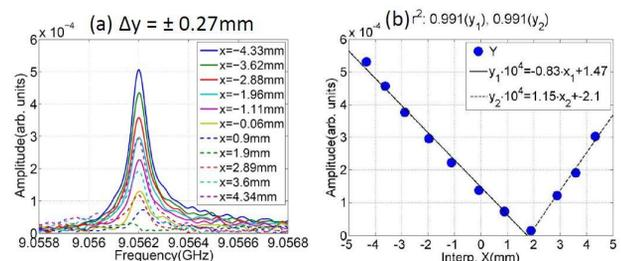
Figure 4: Dipole dependence on transverse beam offset.
