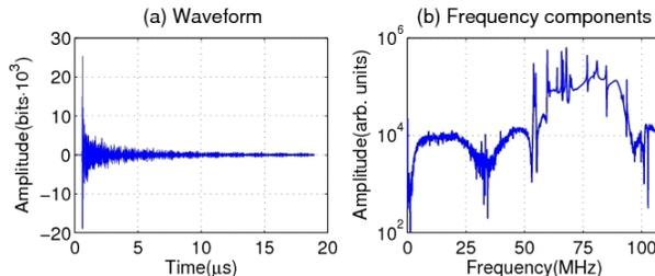
Figure 6: An example waveform and its Fourier transform.
