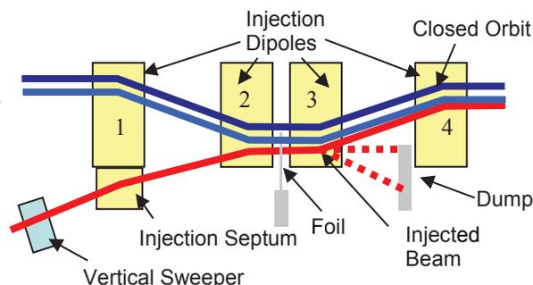
Figure 1: Schematic layout of the existing 70 MeV ISIS injection system.
