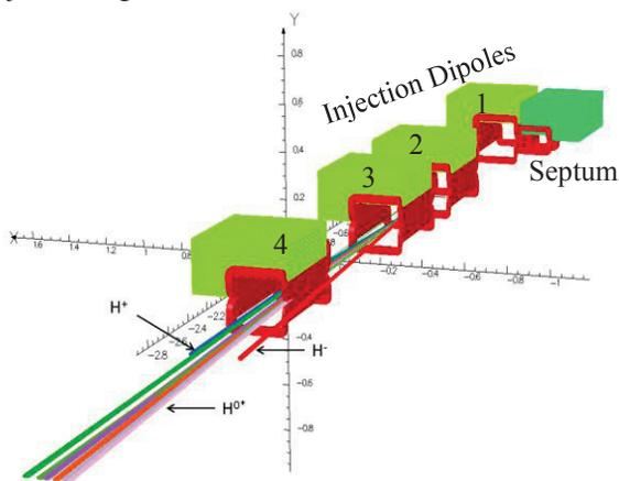
Figure 5: Trajectories for fully, partially, delayed and unstripped particles.
