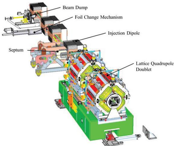
Figure 3: Initial CAD model of the lattice quadrupoles and new injection region.
