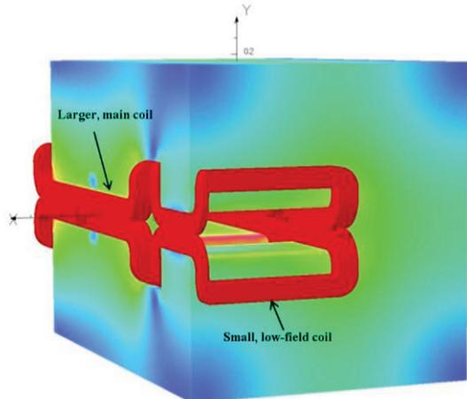
Figure 2. Initial design of a two-stage injection septum.
