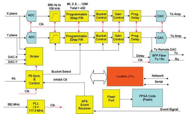
Figure 2: FPGA block diagram of the P0 feedback.
