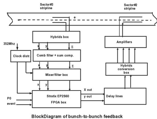
BlockDiagram of bunch-to-bunch feedback
