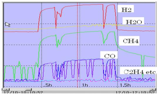
Figure 5: the gas components during the beam operation with high power beam of 300 kW.
