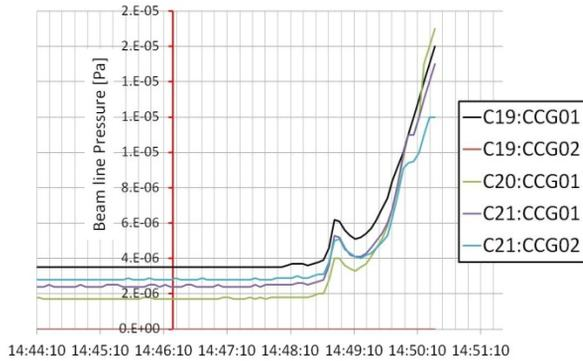
Figure 1: Beam line and fore line pressure at the occurrence of the earthquake.
