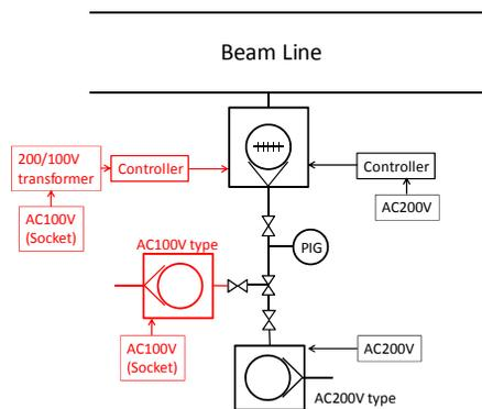
Figure 2: Makeshift pumping system (red ones means) in order to pump with limited electricity.
