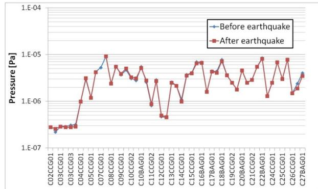
Figure 3: Comparison of beam line pressure distribution after continuous pumping before and after earthquake.
