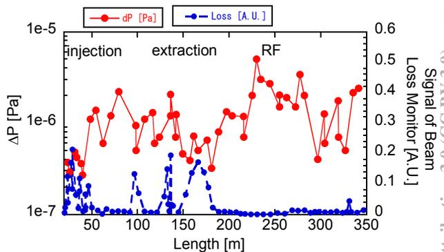
Figure 4: Distribution of beam loss intensity and pressure increase
