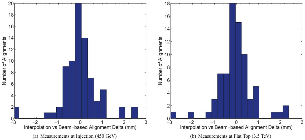
Figure 2: Delta between the BPM-interpolated and the beam-based centers at the LHC collimators in 2011.
