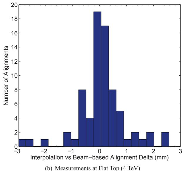
Figure 3: Delta between the BPM-interpolated and the beam-based centers at the LHC collimators in 2012.
