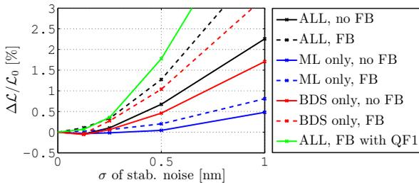
Figure 5: Relative luminosity loss  $\Delta\mathcal{L}/\mathcal{L}_0$  due to white, Gaussian jitter of the corrector actuations in the ML, the BDS and both with a standard deviation  $\sigma$ .
