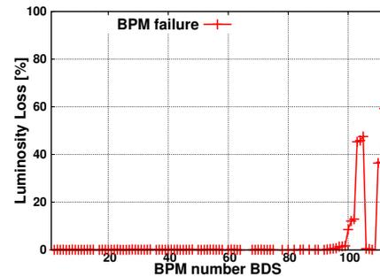
Figure 4: Relative luminosity loss due to a failure of the stabilisation system for an individual BPM in the BDS.
