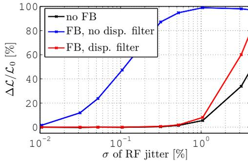
Figure 2: Relative luminosity loss  $\Delta\mathcal{L}/\mathcal{L}_0$  due to white, Gaussian jitter of the acceleration gradients of each decelerator with a relative standard deviation of  $\sigma$ .
