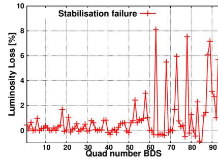
Figure 3: Relative luminosity loss due to a failure of the stabilisation system for an individual quadrupole in the BDS.
