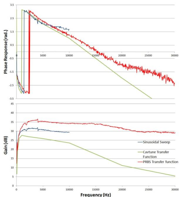
Figure 3: Results of PRBS system identification.
