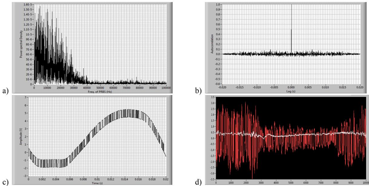
Figure 2: PRBS System Identification up to 30 kHz - a) PRBS autopower function, b) PRBS autocorrelation function, c) Exaggerated PRBS applied to the tuning function, d) Phase detector error from PRBS stimulus (red).
