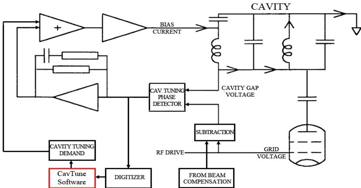
Figure 1: Block diagram of the ISIS Cavity tuning systems.
