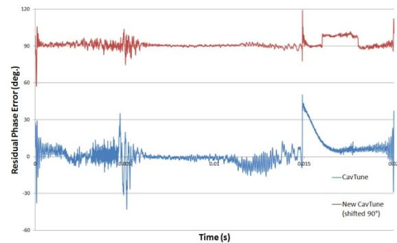
Figure 5: Residual phase error from original and new CavTune software.
