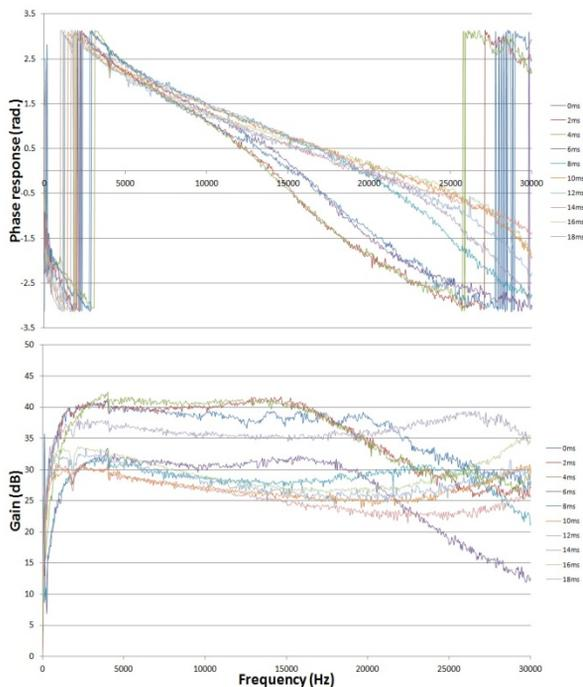
Figure 4: Cavity tuning transfer function variation throughout the acceleration cycle.
