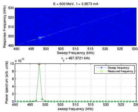
Figure 1: The vertical tune measurement result using the tune scan method. The tune is measured at the energy of 600 MeV with a beam current of 1.2 mA. The span of the sweep is 40 kHz and the bandwidth is 1 kHz, which means that the measurement takes 41 sets of beam signal data in the time domain. The measured vertical tune is 0.1807.
