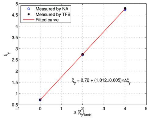
Figure 5: The calibration of the vertical chromaticity knob for the Duke storage ring.
