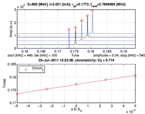
Figure 3: The vertical chromaticity measurement result. The upper plot shows the measured tunes for different energies of the electron beam in the storage ring. The lower plot shows a linear fit to the measured tunes. The slope of the fitted line is used to determine the value of the vertical chromaticity, in this case 0.714.
