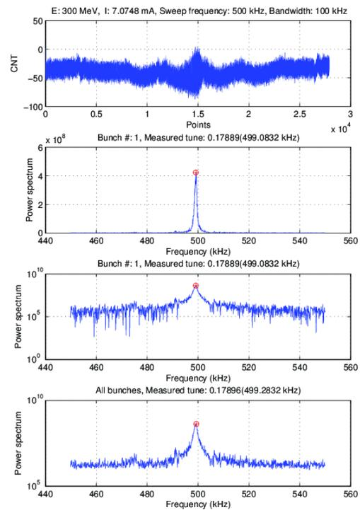
Figure 2: The vertical tune measurement result using the tune monitoring method. The beam is excited by a broadband drive signal with a bandwidth of 100 kHz. The plot on the top shows the overall beam signal in the time domain and the plot on the bottom shows the same signal in the frequency domain. The two plots in the middle show the power spectrum of the bunch signal from bunch #1 in linear scale and in logarithm, respectively. The measured vertical tune is 0.1789.
