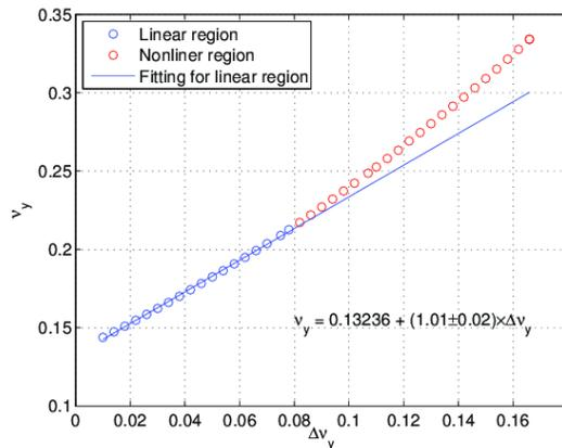
Figure 4: The calibration of the vertical tune knob for the Duke storage ring.
