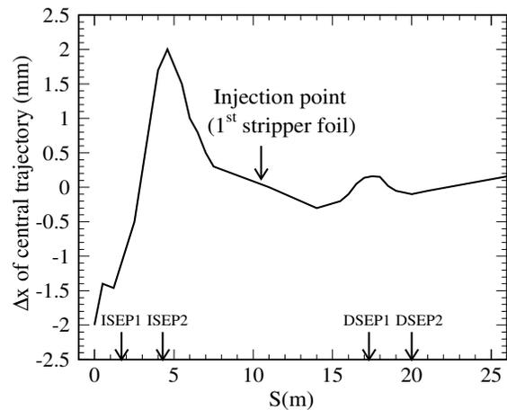
Figure 3: Expected shift of the central trajectory of the injected and the waste beam due to the longitudinal position error of magnets. The shift was within  $\pm 2$  mm and was thus considered to be negligible.
