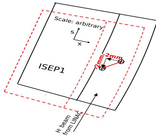
Figure 2: Close view of a typical misalignment of the 1st injection septum magnet. The misalignment in any direction was about -2mm, but it is magnified in the figure by drawing the actual volume of the magnet with arbitrary scales.
