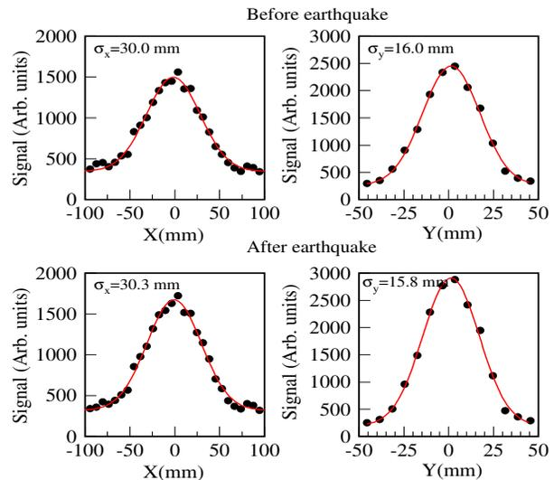
Figure 5: Extracted beam profiles measured after the earthquake (bottom) were found to very identical to those with before the earthquake (top).
