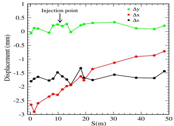
Figure 1: Misalignment of the RCS injection straight section magnets occurred by the earthquake.
