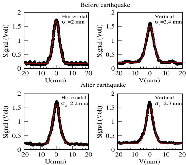
Figure 4: Measured injected beam profiles before (top) and after (bottom) the earthquake were found to be identical.
