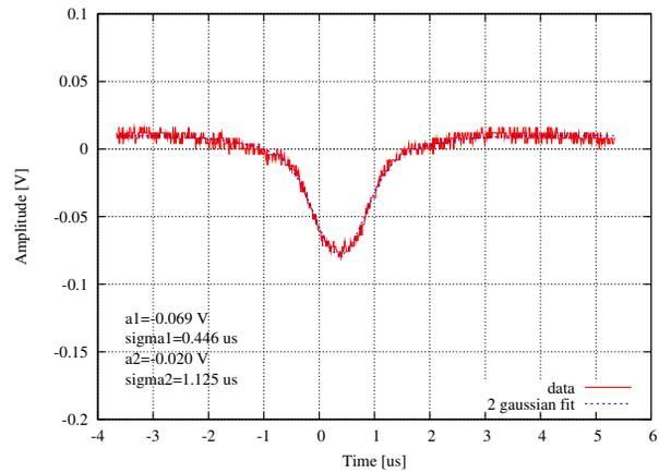
Figure 3: Time domain signal of laser cooled bunched beam observed 60 s after injection. The signal is fitted by two Gaussians. Almost all of the uncooled component was lost, where cooled component still remained.
