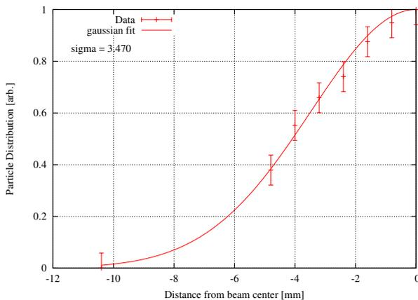
Figure 6: Particle distribution reconstructed from the survival ration measured using the scraper.
