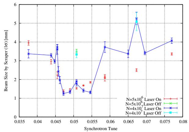
Figure 7: Beam size measurement with a scraper. The betatron tune is (2.052, 1.118).
