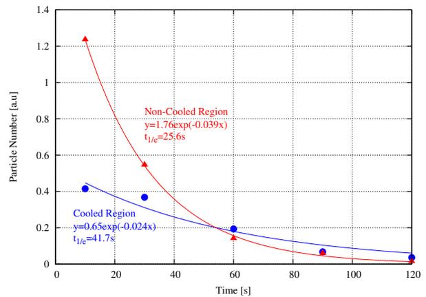
Figure 4: Time evolution of the particle numbers of the cooled and the uncooled region. The lifetime is derived from the reduction rate of particle numbers.
