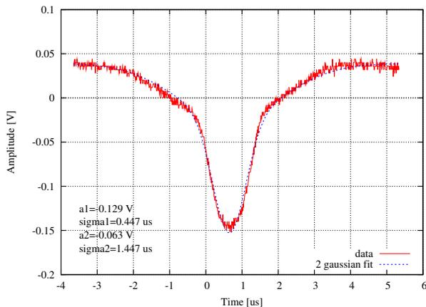
Figure 2: Time domain signal of laser cooled bunched beam observed 30 s after injection. The signal is fitted by two Gaussians.
