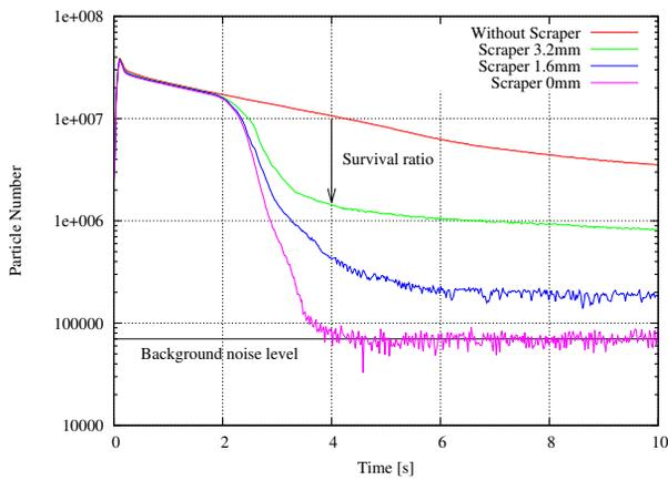
Figure 5: Time evolution of particle number measured by electrostatic pickups. The scraper approaches the beam center within 3.3 s after injection.
