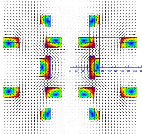
Figure 3: Cross-section of a double half-quadrupole. The coils are wound from simple racetracks in order to facilitate the production in case Nb<sub>3</sub>Sn superconductor technology would be required.
