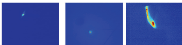
Figure 7: The images of electron beam at the focusing point without pinhole (left) and with pinhole (middle) and at the spectrometer (right).
