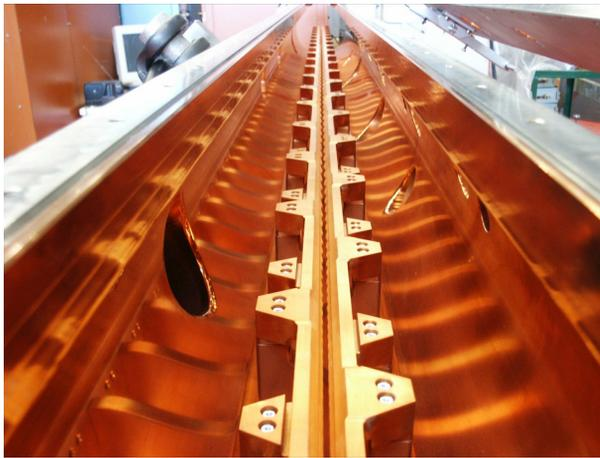
Figure 4: Typical 4-rod-RFQ at 175 MHz.
