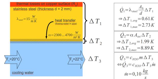
Figure 6: Thermal losses on the copper surface have to be cooled. The calculations are regarding a heat transfer over a 2 mm thick layer of stainless steel. 100 ml/s of water are necessary to cool the sixth stem.
