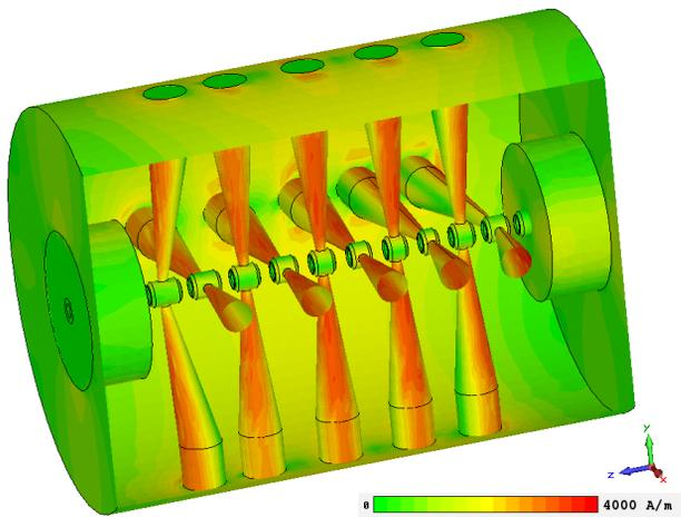
Figure 4: The map of the surface currents on the cavity walls is correlated with the thermal losses [4].
