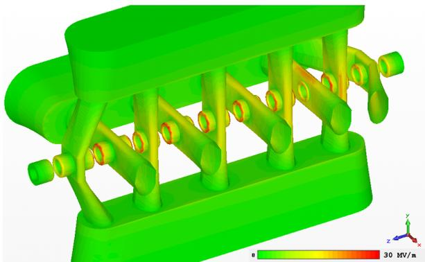
Figure 7: The electric peak fields on the surfaces limit the acceleration gradient. The impact of emitted electrons would cause heat and increase the risk of quenching.
