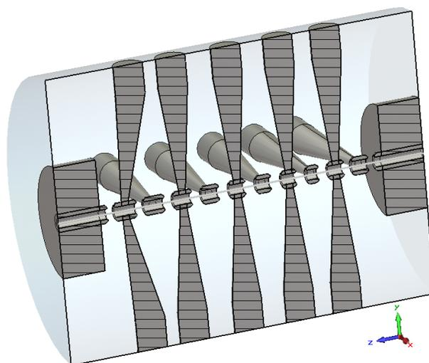
Figure 2: An overview of the first room temperature CH-DTL (MAX – RT CH-1).
