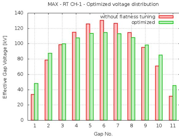
Figure 3: A flat voltage distribution ensures a good heat distribution and therefore a good heat disposal.
