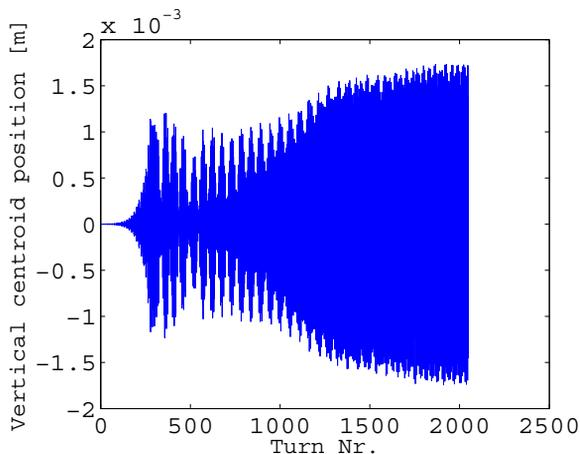
Figure 6: Vertical centroid position of the bunch with  $M = 22$  slices.
