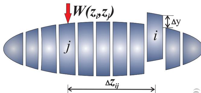
Figure 1: Slicing the 3D bunch in  $M$  longitudinal slices and introducing an offset  $\Delta y$  in the transversal plane for each slice at the time.
