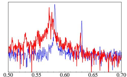
Figure 4: Vertical tune of a single bunch in a train of 100 bunches, measurement (blue) vs. simulation (red) with  $M = 30$  slices.
