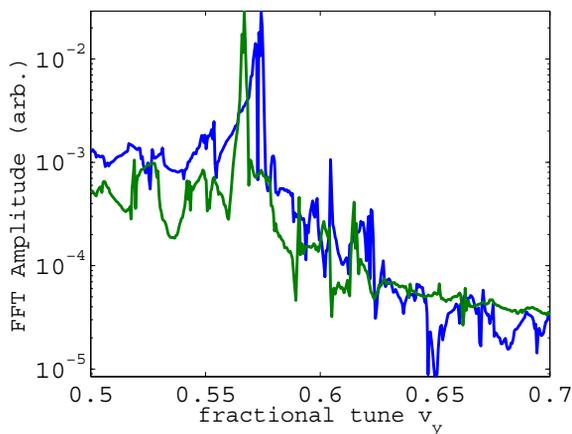
Figure 5: Vertical tune of a single bunch for different number of slices.
