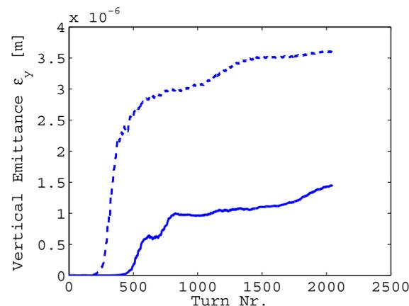
Figure 8: The vertical emittance of the bunch with  $M = 30$  (the solid line) and  $M = 22$  (the dashed line) slices.
