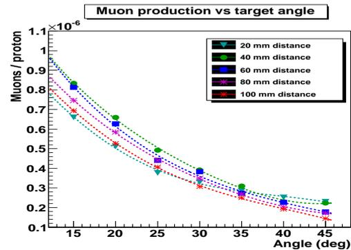
Figure 4: Muon production as a function of target angle for a set of two slabs.
