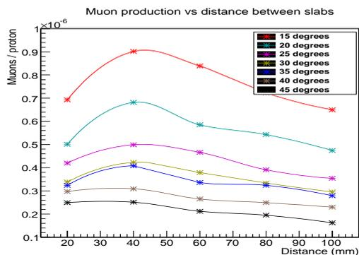
Figure 8: Muons production as a function of slabs distance for a three slabs target geometry.
