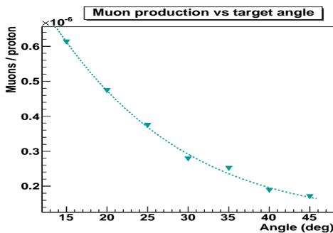
Figure 2: Muon production as a function of the target angle for the original ISIS target.
