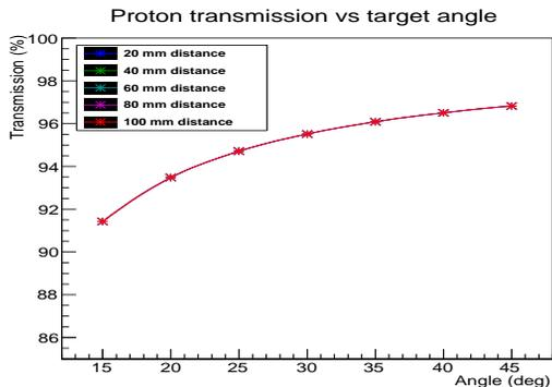
Figure 6: Proton transmission through a set of three slabs.
