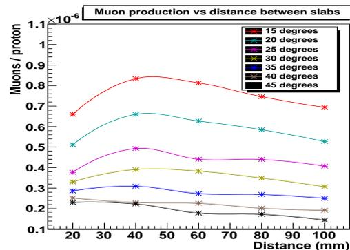
Figure 5: Muons production as a function of slabs distance.
