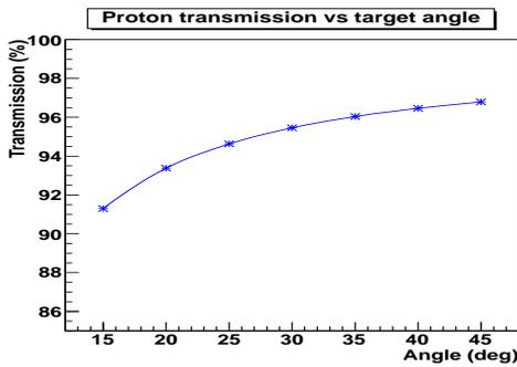
Figure 1: Proton transmission as a function of the target angle for the original target design.
