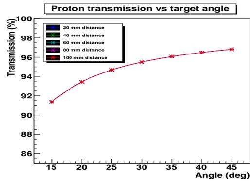
Figure 3: Proton transmission through a set of two slabs of variable orientation angle.
