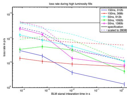
Figure 2: Highest loss rates found in LHC runs with 312, 368, 912, 1092 and 1380 bunches versus BLM signal integration time compared to  $R_{spec} = 4.5 \times 10^{11}$  p/s. The dashed lines show a linear scaling to the nominal number of bunches (2808).
