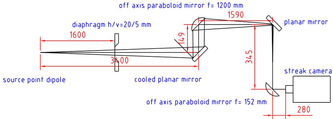
Figure 1: Beam path from the source point inside the bend to the streak camera with the distances shown in mm.
