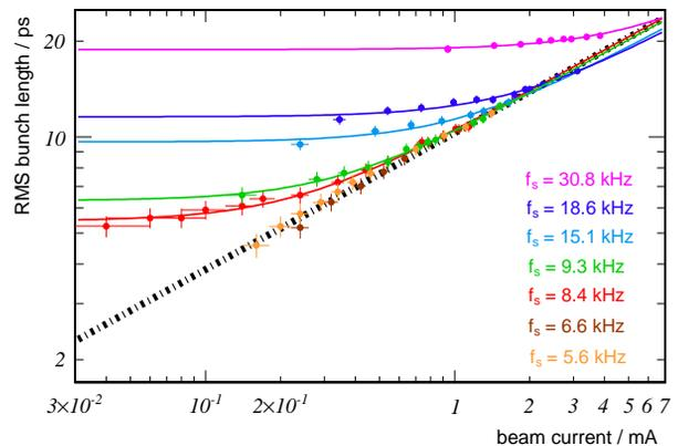
Figure 4: Bunch length as a function of bunch current for different low  $\alpha_c$  optics is visualised. A static uncertainty of  $\pm 2$  pixels on the FWHM of the bunch profiles from which the bunch length data is extracted has been assumed. The dotted black line marks the bursting threshold for ANKA:  $\sigma_z = k \cdot I_{bunch}^{3/7}$  [5] where  $k = 10.3$  for ANKA (for an RF voltage of 0.6 MV). The data set for  $f_s = 8.4$  kHz (red) has been recorded at the new beam port.
