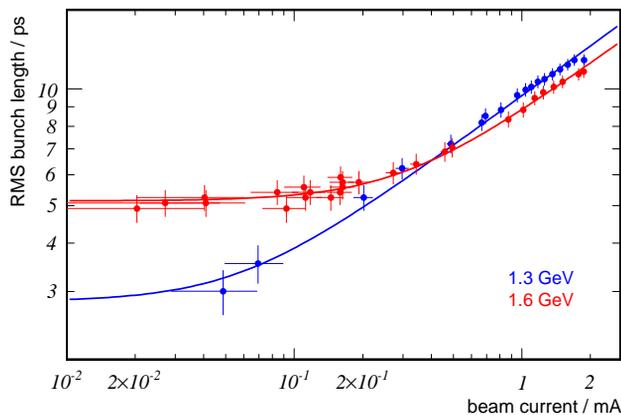
Figure 7: The bunch length as a function of bunch current for different beam energies. The fluctuations in bunch length for currents between 0.1 and 0.2 mA are due to changes in camera settings (slow sweep speed was changed). The RF voltage was set to 1.0 MV (250 kV per cavity). The data for 1.3 GeV is the same as depicted in Figure 6.
