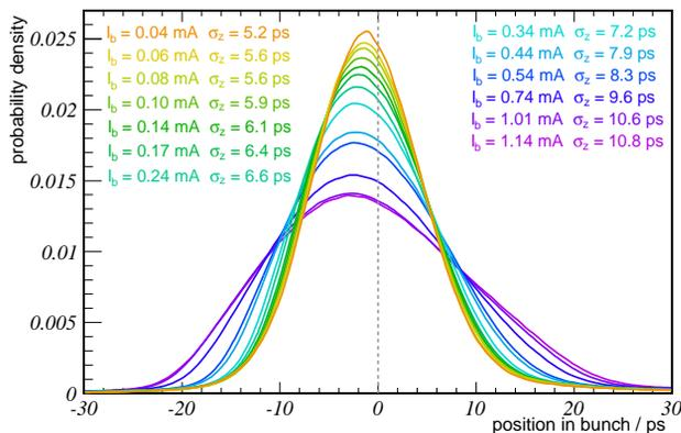
Figure 5: The corresponding bunch profiles for the new data ( $f_s = 8.4$  kHz) from Figure 4.
