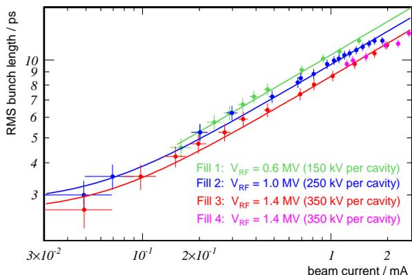
Figure 6: The bunch length as a function of bunch current for different RF voltages at a fixed momentum compaction factor is shown. A static uncertainty of  $\pm 2$  pixels on the FWHM of the bunch profiles from which the bunch length data is extracted has been assumed. The constant factor, but not the exponent of the bursting threshold changes with the RF voltage (leads to an off-set in the logarithmic scale). Bunch lengths as low as 2.7 ps RMS have been measured.
