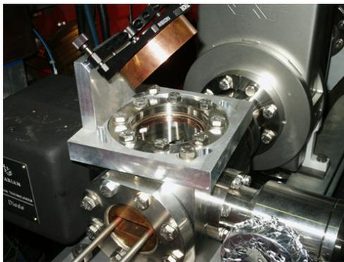
Figure 3: Photon beam exit of the streak beam line front end with cooled mirror, quartz window and parabolic mirror. The set up is covered by a lead box (removed).
