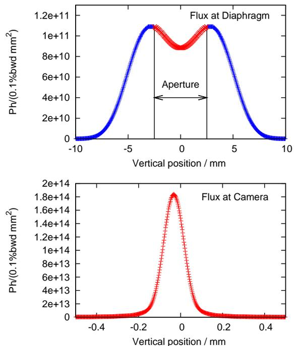
Figure 2: Top: Simulated photon flux at the diaphragm in dependence of vertical position. The part marked in red between -2.5 and 2.5 mm can pass through the aperture, the rest is absorbed. Bottom: Simulated photon flux at the focus point where the streak camera is placed.
