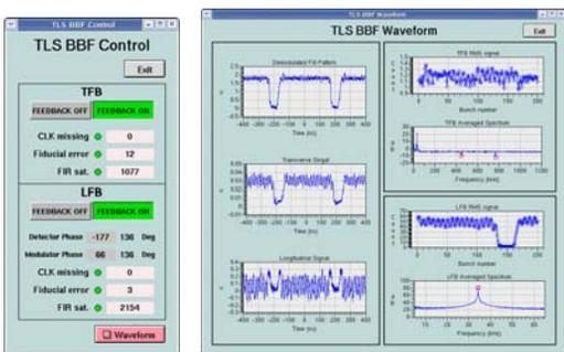
Figure 1: Operator interface to operate the bunch-by-bunch feedback system includes of transverse as well as longitudinal feedback system. Various waveforms include of filling pattern, beam oscillation amplitude in RMS and bunch phase oscillation in RMS, are shown on the integrated with front-end and iGp control page. Corresponding spectrum are shown also, it is easily used as a tune monitor.
