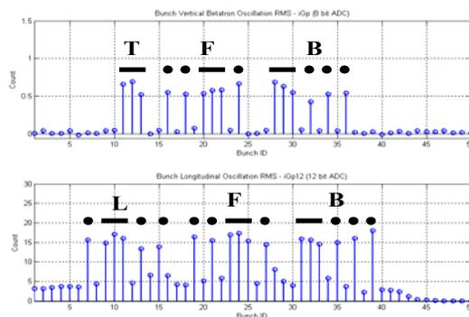
Figure 4: Bunch oscillation amplitude due to selective bunches excitation. The excite pattern of “TFB” and “LFB” are encoded by Morse code.
