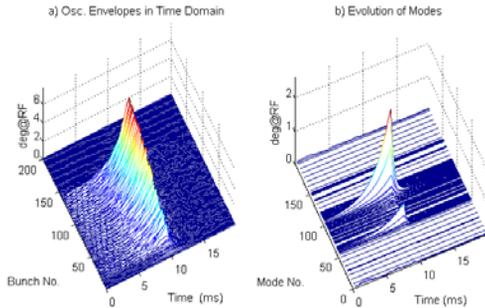
Figure 5: Typical growth-damp data in longitudinal feedback loop..
