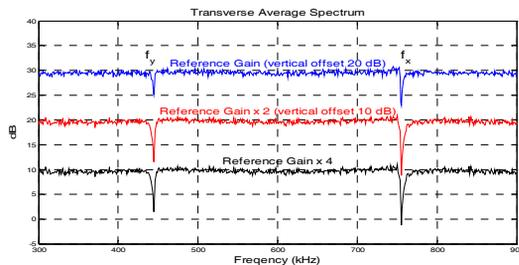
Figure 3: Tune measurement by extract the notch position in the bunch averaged spectrum when feedback loop is activated.
