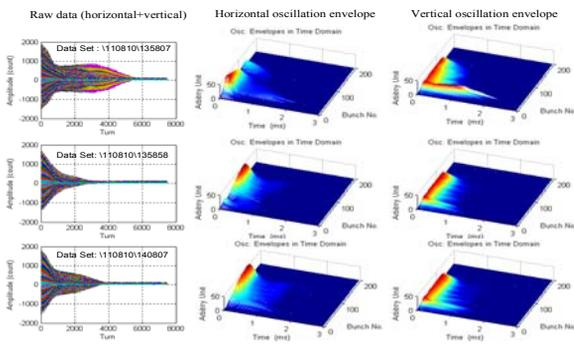
Figure 6: Stored beam perturbation due to kickers at injection instance.
