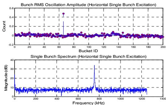
Figure 2: Single bunch excitation and single bunch spectrum for tune identification.
