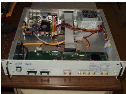
Figure 2: The iGp-12 feedback unit including 12bit ADC and DAC, Xilinx Virtex-5 FPGA, a Mini-ITX motherboard with a solid-state drive.
