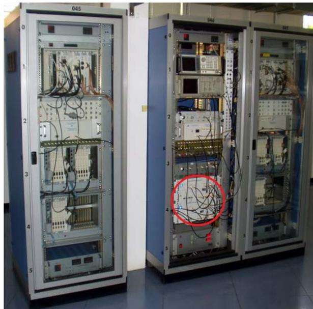
Figure 1: Three racks with the previous version of the longitudinal feedback electronics and the new one circled in red.
