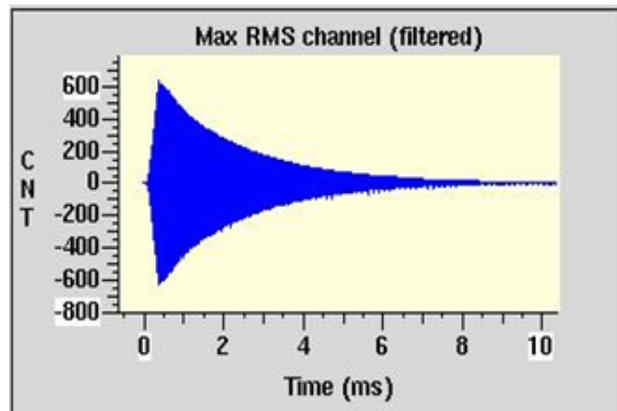
Figure 3: Vertical decoherence measurements, obtained by exciting the beam with the vertical feedback.
