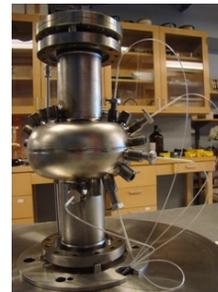
Figure 3: Single cell experimental setup for optical emission spectroscopy.
