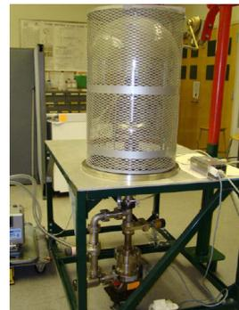
Figure 1: Single cell cavity experimental setup.
