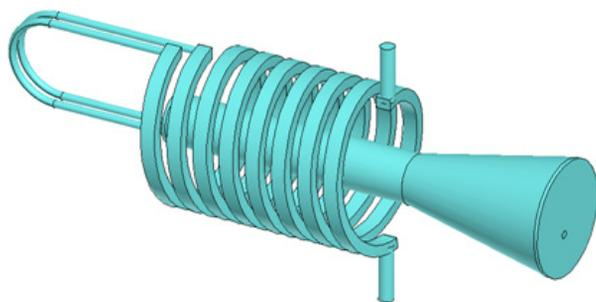
Figure 6: Schematic drawing of cooling channel at the RF input coupler tip
