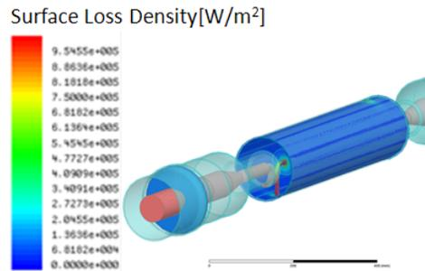
(c) Surface loss density of the coupling cavity loop
