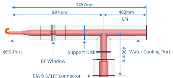
Figure 1: Schematic drawing of an RF input coupler with water cooling port of  $\lambda/4$
