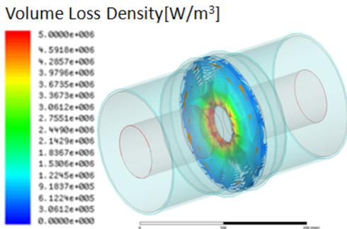
Figure 3: Volume loss density of  $\text{Al}_2\text{O}_3$  ceramics
