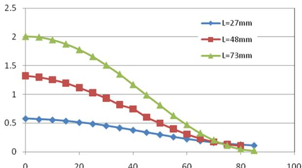
Figure 5: Evaluation for beta (RF coupling) on beam in IFMIF/EVEDA RFQ; beta vs. loop angle
