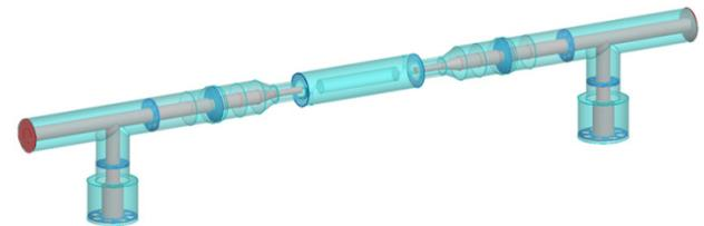
(a) RF transmission power test system
