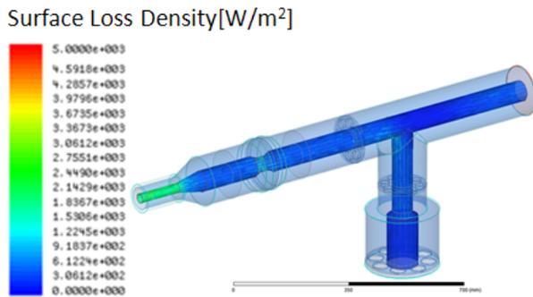
Figure 2: RF loss density of the RF input coupler
