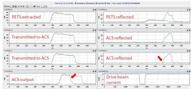
Figure 6: A breakdown in the ACS detected by cut in the output signal and rising of the reflected power.
