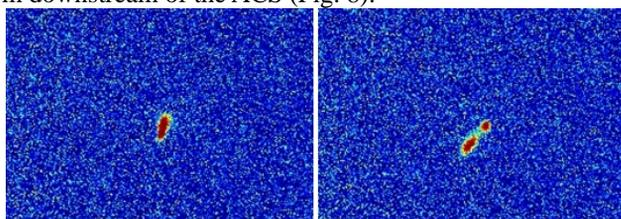
Figure 8: Beam profile without (left) and with (right) breakdown.
