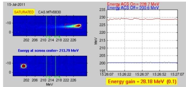
Figure 4: Spectrometer screen with tracking of accelerated (up) / not accelerated (down) beam.
