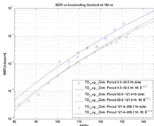
Figure 7: Breakdown rate vs. accelerating gradient for various periods of conditioning.
