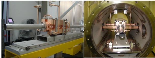
Figure 3: ACS in its vacuum tank.
