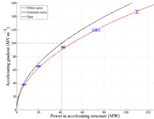
Figure 5: Accelerating gradient vs. RF power.
