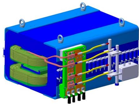
Figure 4: Transfer-line bending magnet.
