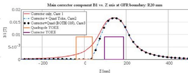
Figure 3: Influence of the adjacent quadrupole on the field distribution on the corrector.
