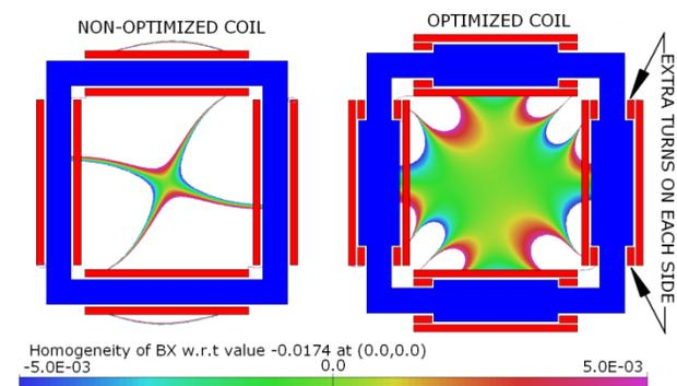
Figure 2: Non-optimized vs. optimized coils.
