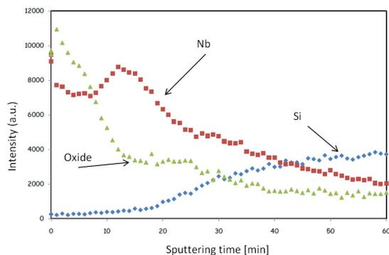
Figure 3: Depth profile of the XPS measurement. One can clearly see the Nb oxide layer at the surface, while the oxygen content decreases with deepness. Looking at the raw data it can clearly be seen that there is an oxygen peak appearing at the interface between the Nb thin film and the substrate.
