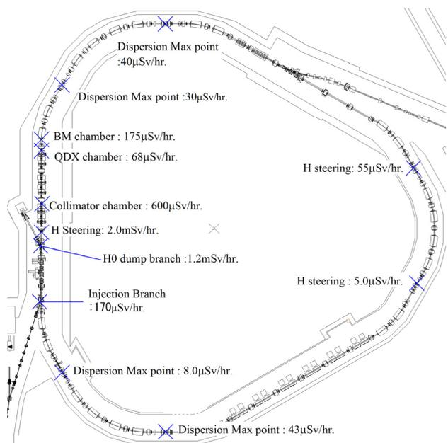
Figure 3: Residual dose distribution after 300kW operation.
