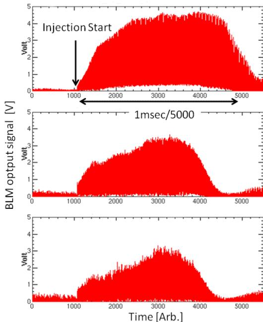
Figure 2: BLM signal at the H0 dump branch. Upper figure shows the BLM signal without painting. Middle figure shows the BLM signal with 100πmm-mrad painting. Lower figure shows the BLM signal with 150πmm-mrad painting.
