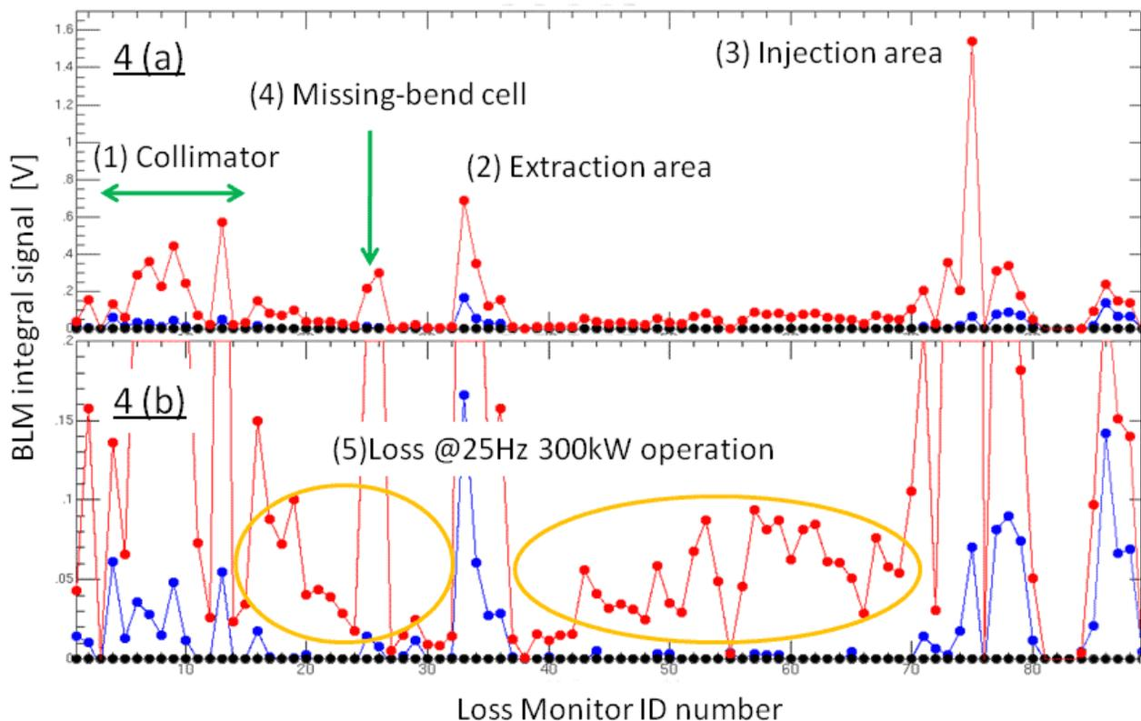
Figure 4: The integrated BLM signals around the RCS beam line. The BLM signals were integrated during acceleration period (20msec). Horizontal axis is the ID number of the BLMs. Blue line is the BLM signals at 120kW and Red line is the BLM signals at 300kW.
