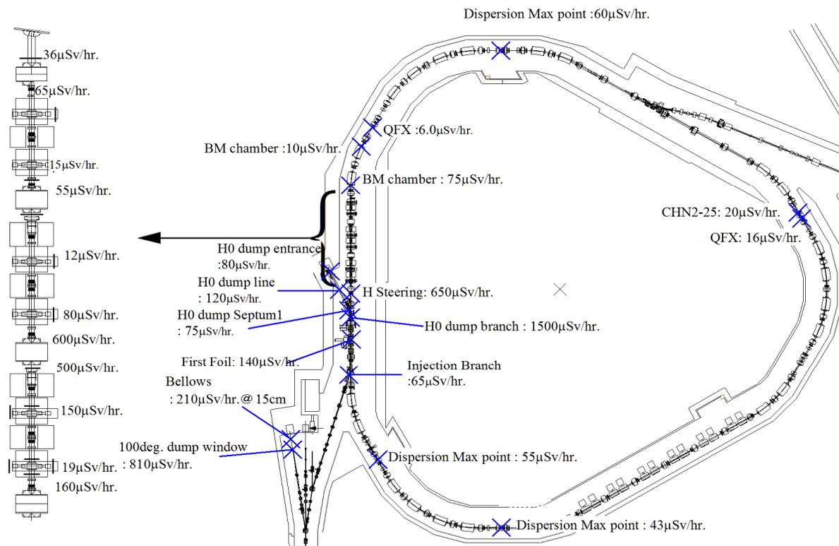
Figure 1: Residual dose distribution after 120kW operation.
