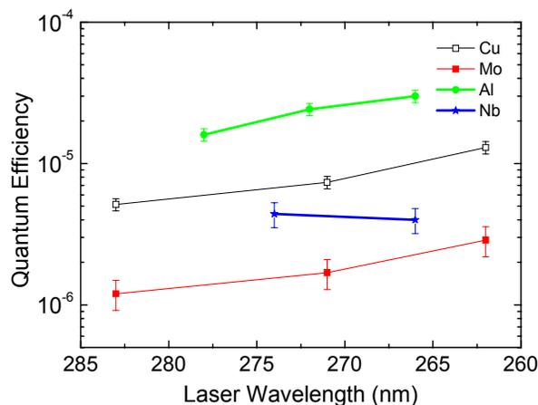
Figure 6: Quantum efficiency measurements for various cathode material at different laser wavelengths.
