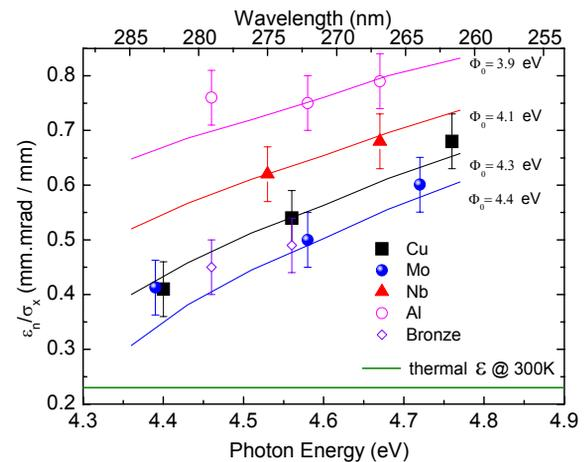
Figure 5: Normalized intrinsic emittance/mm for different cathode materials versus photon laser energy with theoretical curves according to eq (1).
