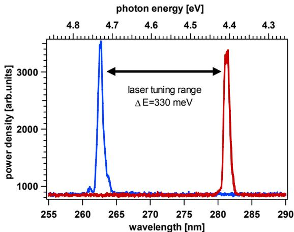
Figure 3: Wavelength tuning range of the frequency-trippled Ti:sapphire laser.
