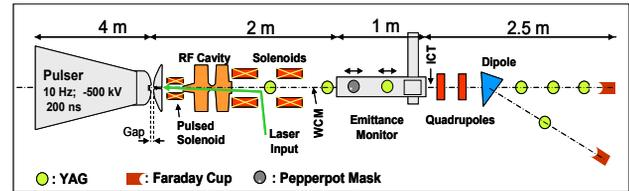
Figure 4: Schematic of the Diode-RF gun and the 4 MeV accelerator beam line with diagnostics
