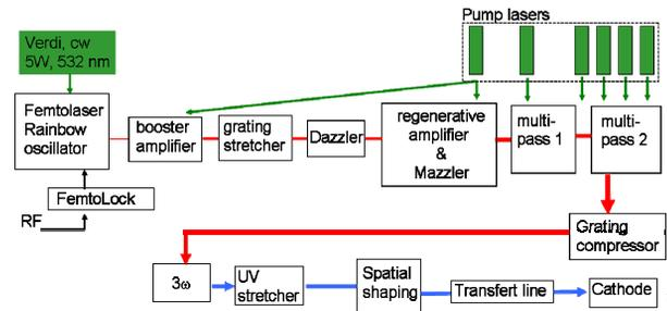
Figure 1: Amplifier layout with 3<sup>rd</sup> harmonic generation.
