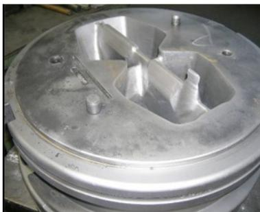
Figure 1: The extrusion die.
