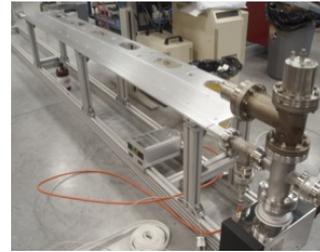
Figure 6: A chamber during RGA scan and vacuum test
