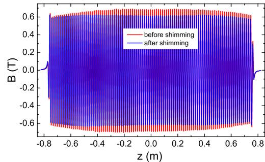
Figure 2: Field profile measured at 135 A before ( $g = 7.75$  mm, red) and after mechanical shimming ( $g = 8.25$  mm, blue).
