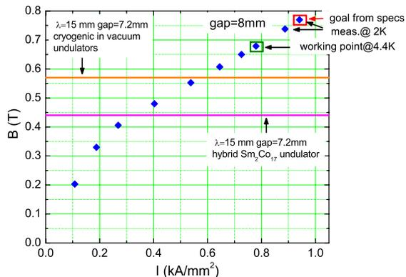
Figure 3: Measured peak field at 7.75 mm and 8.25 mm as a function of engineering current density rescaled to the 8 mm gap.
