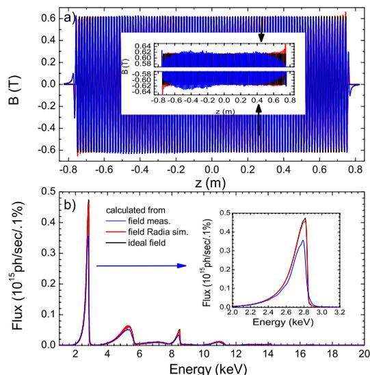
Figure 4: a) Field profile measured at 135A and gap=8.25 mm (blue), simulated with Radia with the pole heights and half period lengths measured on the magnet at room temperature (red), and ideal (black). In the inset are shown the positive and negative field peaks along the magnet. b) Flux calculated with B2E [6] using the three above fields through a slit of 1mm x 1mm at 10 m distance from the middle of the undulator. In the inset the first harmonic is zoomed.
