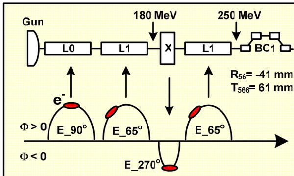
Figure 1: Linac layout up to BC1 and beam compression process.
