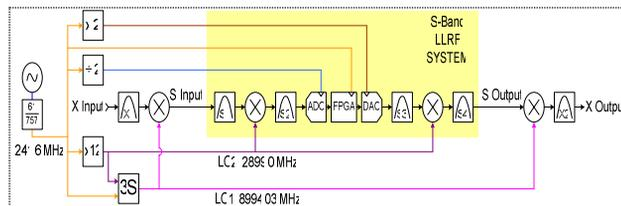
Figure 5: X-band LLRF system layout with the S-band system yellow shaded.
