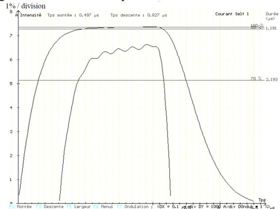
Figure 3: Pulse shape estimation of the PFN with a total external inductance of 2.0  $\mu\text{H}$ .
