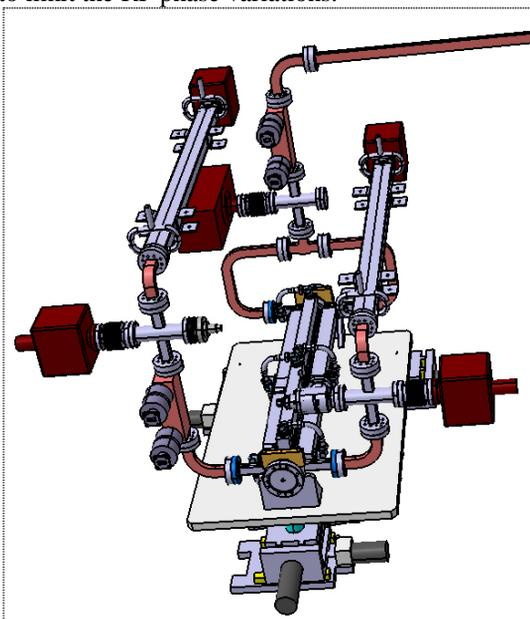
Figure 4: Accelerating structure and WG connections.
