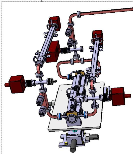
Figure 4: Accelerating structure and WG connections.
