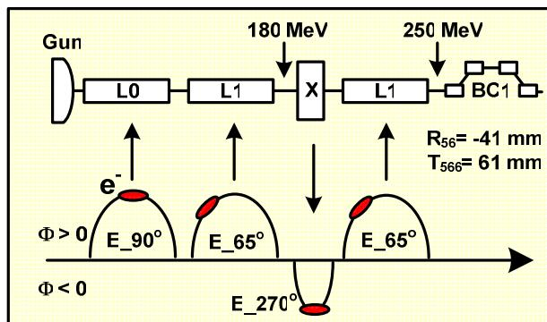
Figure 1: Linac layout up to BC1 and beam compression process.
