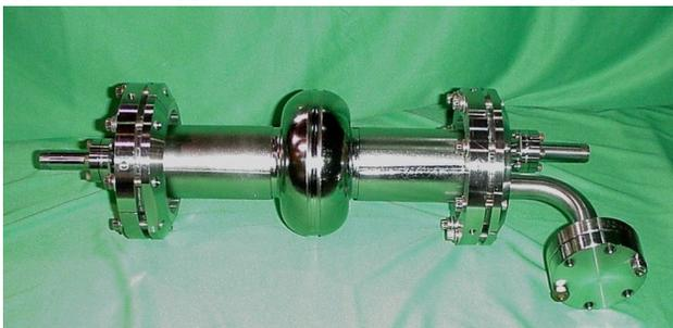
Figure 1: 2.45 GHz niobium cavity for the cold (2K) test.
