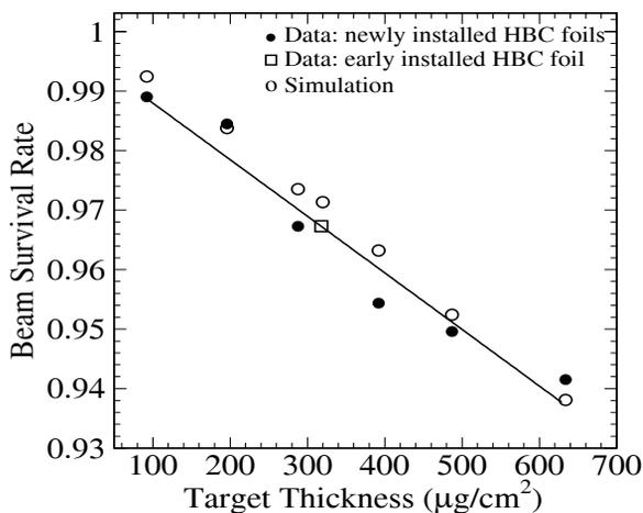
Figure 3: A comparison of the measured and simulated beam survival rate at the end of 500 turns are shown. Thickness of the earlier installed HBC foil is determined by using a linear fitting of the data measured with six newly installed HBC foils together with the data measured with that particular foil as shown by an empty square symbol.
