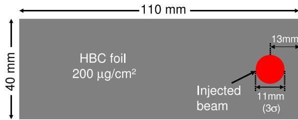
Figure 2: Typical stripping foil size and thickness in RCS. Foil edge to the injection beam center was kept 13 mm for the present study.
