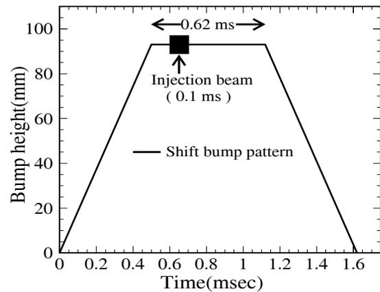
Figure 1: Shift bump pattern and the injection beam timing set for the present study. In order to measure the beam loss with good accuracy, the circulating beam hitting time on foil was intentionally increased by keeping the shift bump constant at-top for further 420 ms after the injection.
