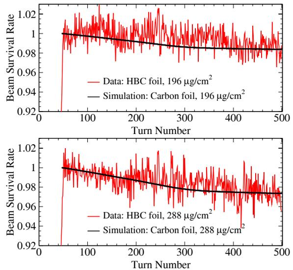
Figure 4: Comparisons of the measured and simulated turn-by-turn beam survival rates are shown for two targets with different thickness. The global shapes are found to be consistent with each other.
