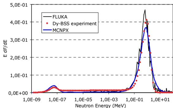
Figure 3: Experimental and computational neutron spectra in the point of test at 150 cm from the target at  $90^\circ$  wr to the impinging electron beam line.
