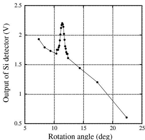
Figure 2: X-ray measurement with rocking curve method.
