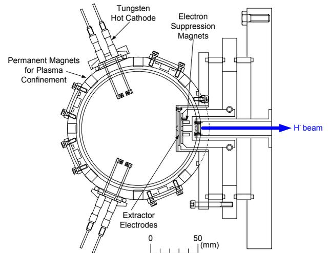
Figure 3: A schematic drawing of an  $H^-$  ion source for a negative ion beam probe system.
