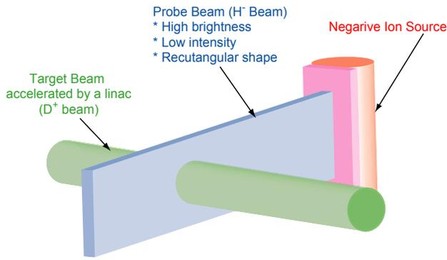
Figure 1: A conceptual drawing of the negative ion beam probe system.
