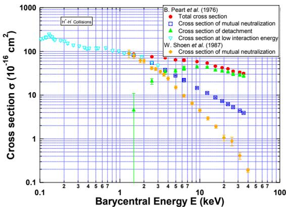
Figure 2: Cross section of electron detachment from  $H^-$  by  $H^-+H^+$  collisions in low energy regions.
