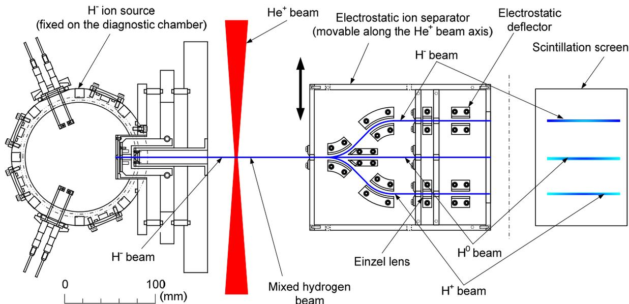
Figure 4: A schematic drawing of the experimental set up of the  $H^-$  beam probe system to monitor the beam profile of the high current density  $He^+$  beam extracted from an extraction system with three concaved electrodes.
