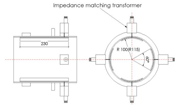
Figure 2: BPM head for the 3-50 BT.
