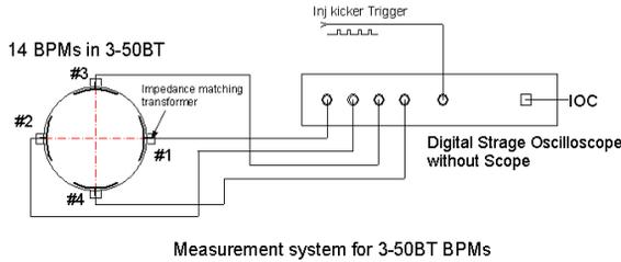
Figure 3: Schematic of the BPM system for the 3-50 BT.
