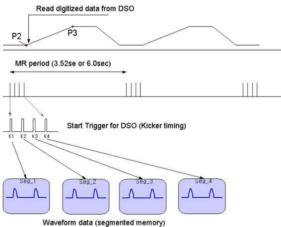
Figure 4: Time chart for segmented memory acquisition.
