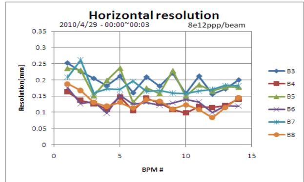
Figure 7: Distribution of all horizontal resolutions of the BPMs in the 3-50 BT.
