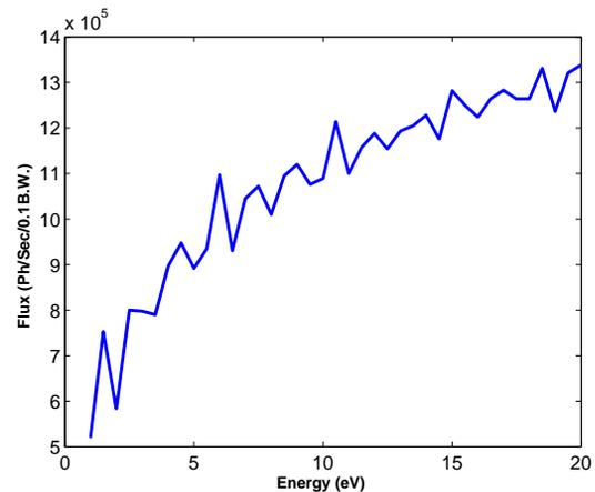
Figure 2: ORS undulator spectrum
