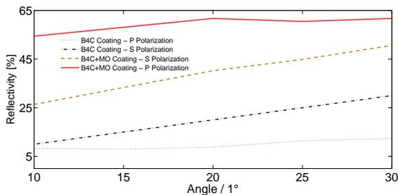
Figure 3: Reflection of GI mirrors for IR laser
