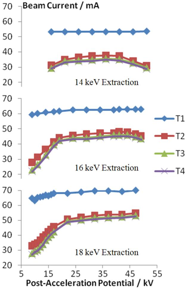
Figure 3: Effect of post-acceleration on beam transport.
