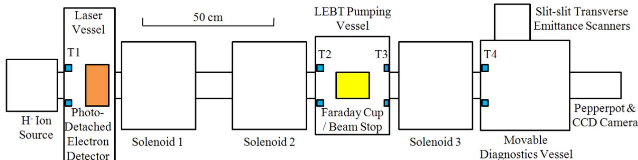
Figure 1: Present FETS diagnostics equipment, shown to scale. Labels T1-4 denote beam current transformer toroids.
