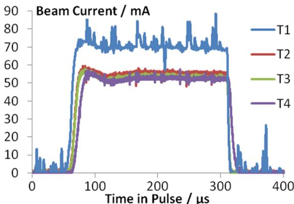
Figure 4: Beam currents measured in the four LEBT toroids at design beam energy and solenoid settings.
