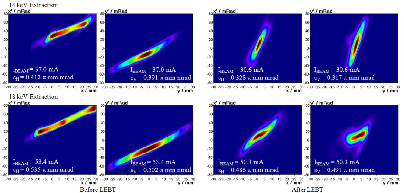
Figure 2: Horizontal and vertical emittance plots before (left pairs) and after (right pairs) the LEBT solenoids for extraction energies of 14 keV (top row) and 18 keV (bottom row). The post-acceleration potential applied was 24 kV.
