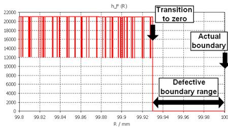
Figure 1:  $H_\varphi(r)$ , cavity radius  $R$ : 100 mm, method: FIT. FEM-computed fields have a significantly smaller defective boundary range ( $0.3 \mu\text{m}$ ) than the shown FIT-computed ones ( $70 \mu\text{m}$ ) which are allocated on the dual grid in a certain distance to the boundary.
