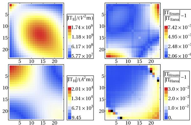
Figure 6: Absolute values and relative error of the  $IT_E$  and  $IT_H$  for radial perturbation of 5% using  $3.4 \cdot 10^5$  cubic volume elements with 0.5 mm step size. For two  $IT_H$  that are almost zero the error is not shown (black areas).
