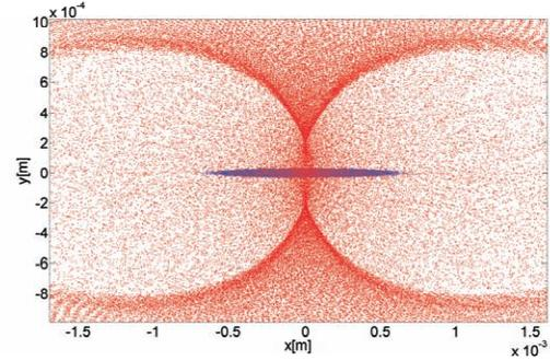
Figure 2: Transversal profile of the ILC bunch (blue dots) and the e-cloud (red dots) after the bunch passes through the cloud.
