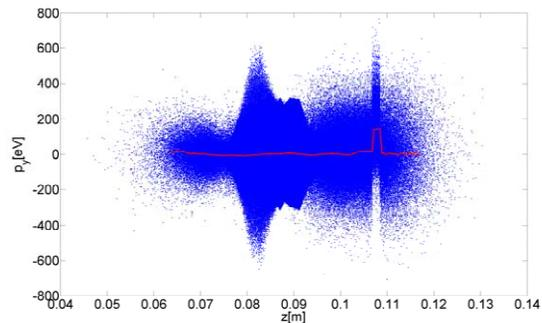
Figure 6: Transversal impulse ( $p_y$ ) of the ILC bunch particles from Figure 5 after the passage through the e-cloud.
