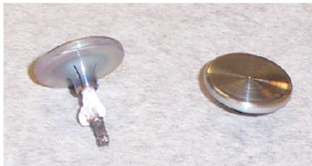
Figure 3: Melted feed-through of a lower button and the fallen upper button.
