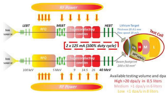
Figure 1: Schematic of IFMIF.
