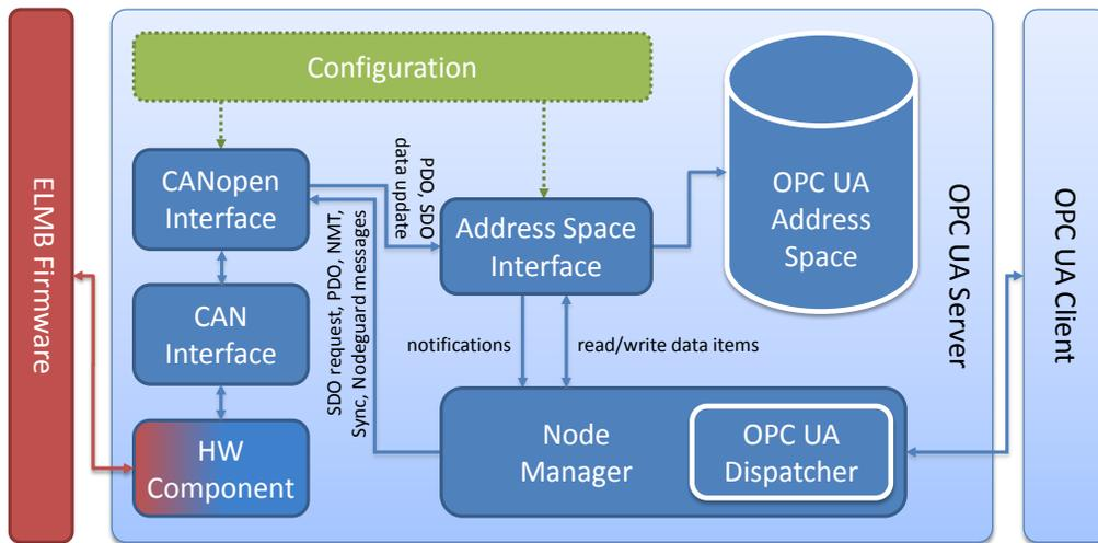
Figure 2: Software components of the server and data flow among them. CANopen specific terms like SDO, PDO, NMT are described in [2].
