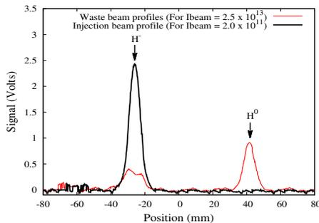
Figure 4:  $H^0$  and  $H^-$  (if any) components of the waste beam can be measured simultaneously by the MWPM7.
