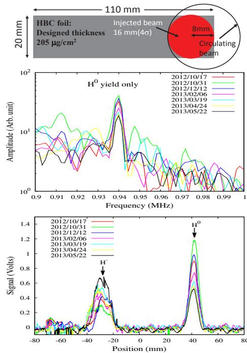
Figure 5: A continuous reduction of the  $H^0$  yield during 7 months operation is measured by both H0CT and the MWPM7 reflecting an increase of the foil thickness. There was significant amount missing  $H^-$  due to 20 mm vertical size of the primary stripper foil as demonstrated at the top.
