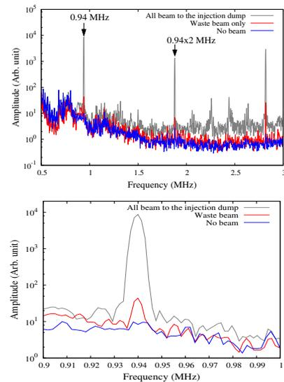
Figure 3: Fourier transform of the HOCT time domain data clearly shows the beam signal. The difference of the waste beam signal (red) from the no beam (blue) can be clearly seen in the expanded view (bottom). The spectrum shown in gray color is taken in the injection beam dump mode.
