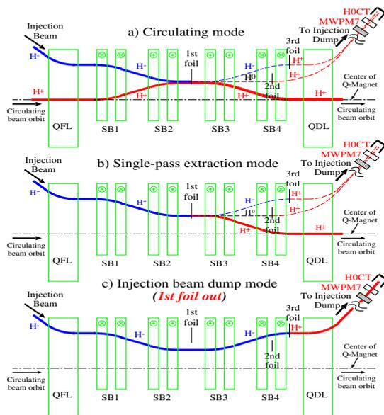
Figure 1: Close view of the RCS injection area and location of the HOCT and MWPM7. A ratio of the beam signal measured by mode (a) or (b) to that of mode (c) gives the waste beam fraction.
