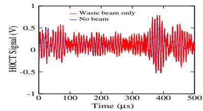
Figure 2: Time domain signals of the HOCT with beam (red) and with no beam (blue) are quite identical and is hard to extract the real information of the waste beam.
