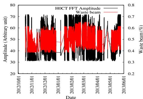
Figure 7: Online trend of the H0CT for the waste beam fraction is found to be similar to that measured several times as shown in Fig. 6 and was about 0.5% in average.
