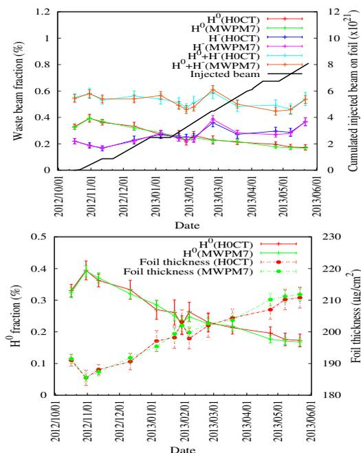
Figure 6: Individual  $H^0$  and  $H^-$  waste beam fractions and their sum for 13 measurements during 7 months operation. The integrated injected beam is shown by the black curve. The corresponding foil thickness is shown in the bottom.
