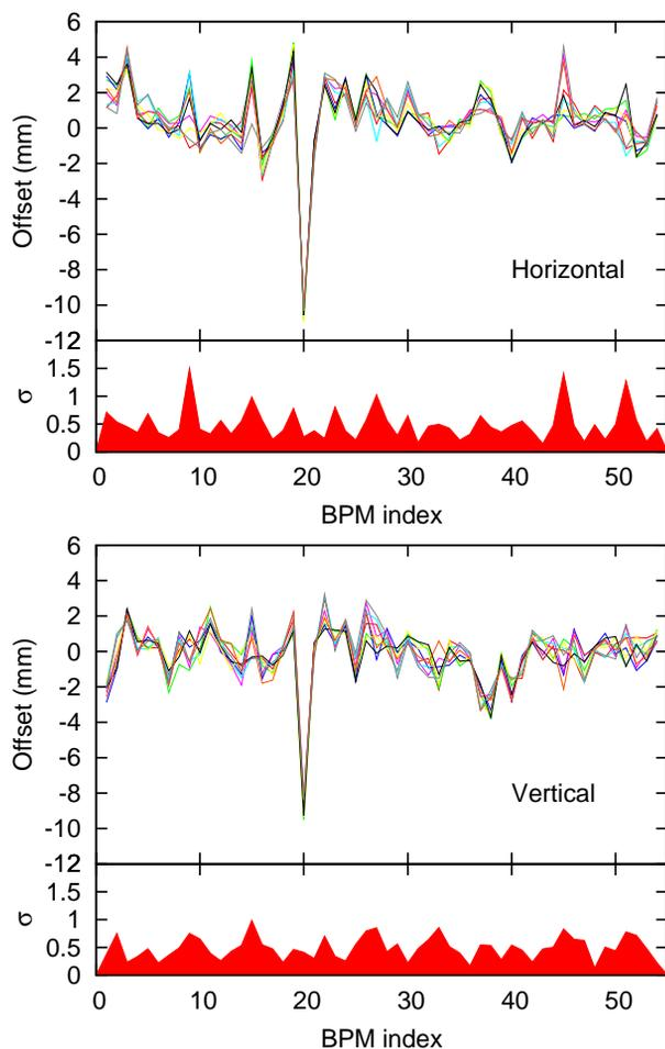
Figure 4: Results of estimated offset for all 54 BPMs. Nine different initial orbits are plotted with several colors. The upper plot contains results for horizontal and the lower plot is for the vertical offset. The bottom bands indicate the estimated error for each BPM.
