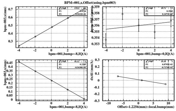
Figure 1: Example of MR BBA. Three plots show the position changes as a function of the auxiliary coil current. The right down graph indicates the determination of the BPM offset.
