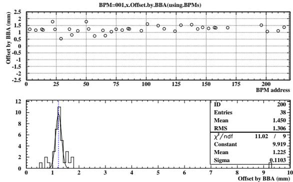
Figure 2: BPM001 offset determination by whole BPM around the ring. Upper shows determined offset values by individual BPM. Lower shows statistics of all BPM results.
