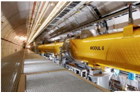
> TESLA type superconducting accelerating modules 1.3 GHz
