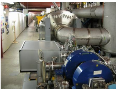
> Normal conducting 1.3 GHz RF gun > Ce 2 Te cathode > Two Nd:YLF based ps photocathode lasers
